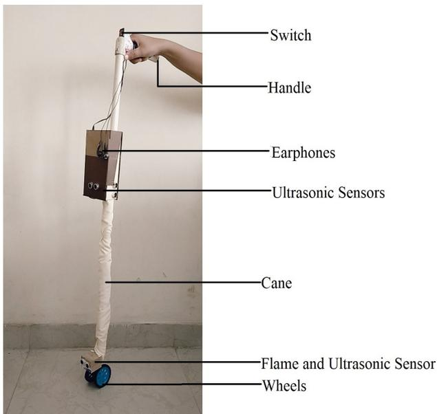
Fig-11: Smart Cane for visually impaired
