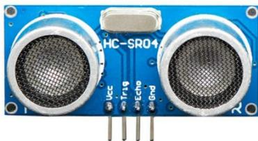
Fig-5: Ultrasonic Sensor HC
